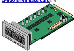
This card is only supported in an IP500 V2 control unit running in IP Office Basic Edition - PARTNER® Mode or IP Office Basic Edition. It provides 6 ETR ports for connection of ETR phones. 2 Analog extension ports are also provided for emergency use only with an analog trunk
