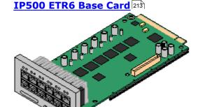
This card is only supported in an IP500 V2 control unit running in IP Office Basic Edition - PARTNER® Mode or IP Office Basic Edition. It provides 6 ETR ports for connection of ETR phones. 2 Analog extension ports are also provided for emergency use only with an analog trunk card
